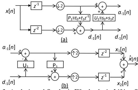
Fig. 3: Analysis and Synthesis Filterbanks in Lifting Steps
