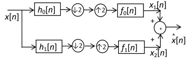
Fig. 2: Two Channel Biorthogonal Wavelet System
