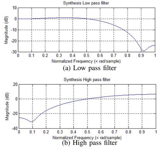
Fig. 4: Frequency response of synthesis end filters
