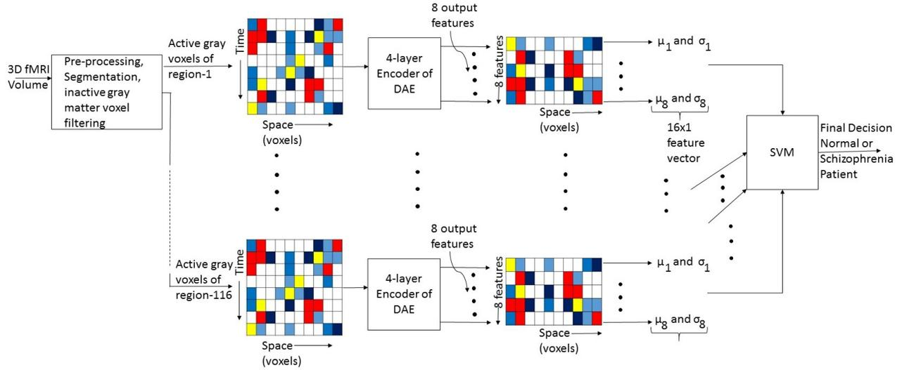
Figure 3: Proposed Two Stage Architecture
