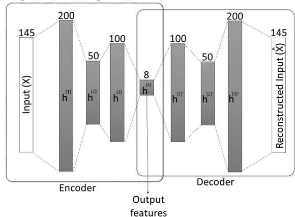
Figure 2: Architecture of Stacked Auto Encoder
